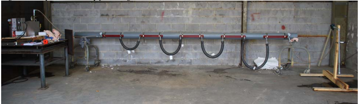
Figure 2: Experiment set-up featuring boiler, ControTrace, and ten JIC connections.
