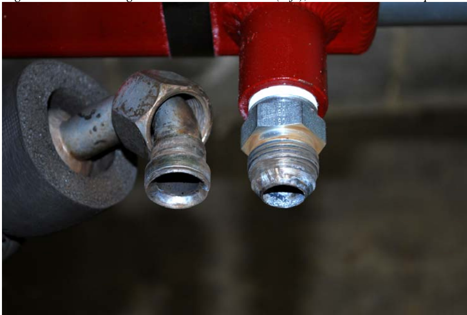
Figure 1: FJIC tubing connection on hose end (left); MNPT X MJIC adapter on jacketing (right)
