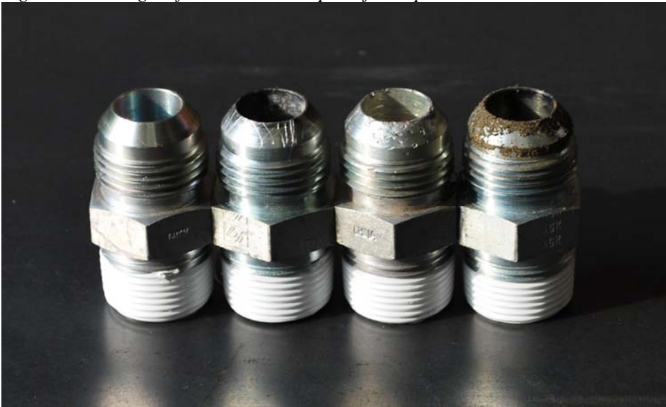
Figure 4: Damage inflicted to JIC adapters for Expts 10-11.
