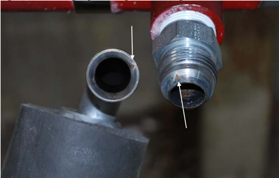
Figure 3: JIC sealing surface damage caused during 12-hour leak test.
