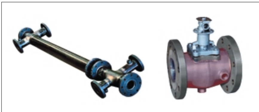
Fig. 5: Spools of jacketed sulphur piping. Note the multiple crosses for rodding out the lines.
