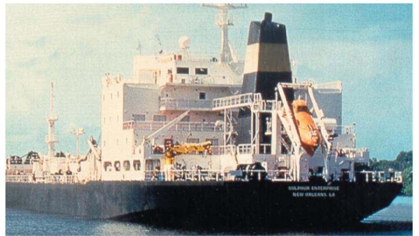
TOP: The M/V Sulphur Enterprise carries about 24,000 tons of molten sulphur from Louisiana and Texas to Florida. A sophisticated thermal maintenance system with bolt-on heating elements from Controls Southeast Inc. keeps the molten cargo flowing for loading and discharge.
