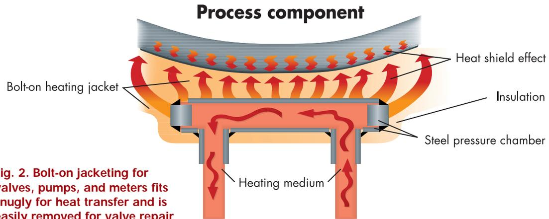
**Fig. 2. Bolt-on jacking for valves, pumps, and meters fits snugly for heat transfer and is easily removed for valve repair or changeout.**
