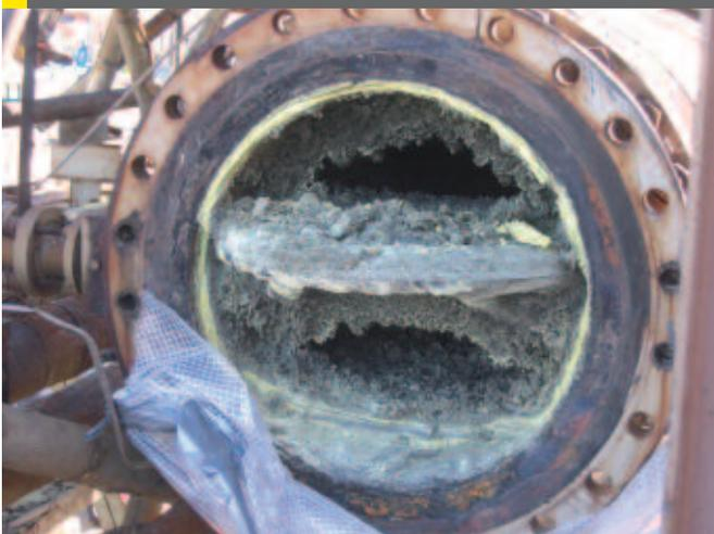
**Fig 2: Tail gas line failure due to extreme corrosion**
