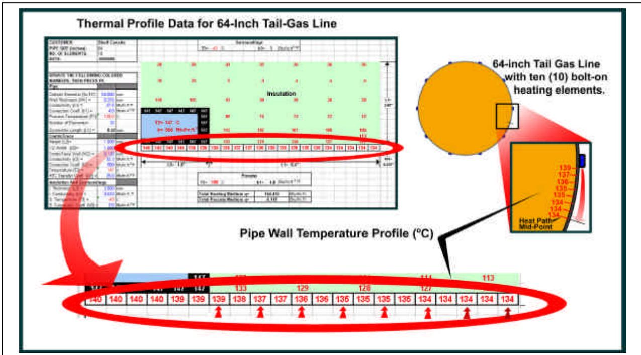
FIGURE 9 THERMAL MODELING DATA WITH PIPING TEMPERATURE PROFILE
