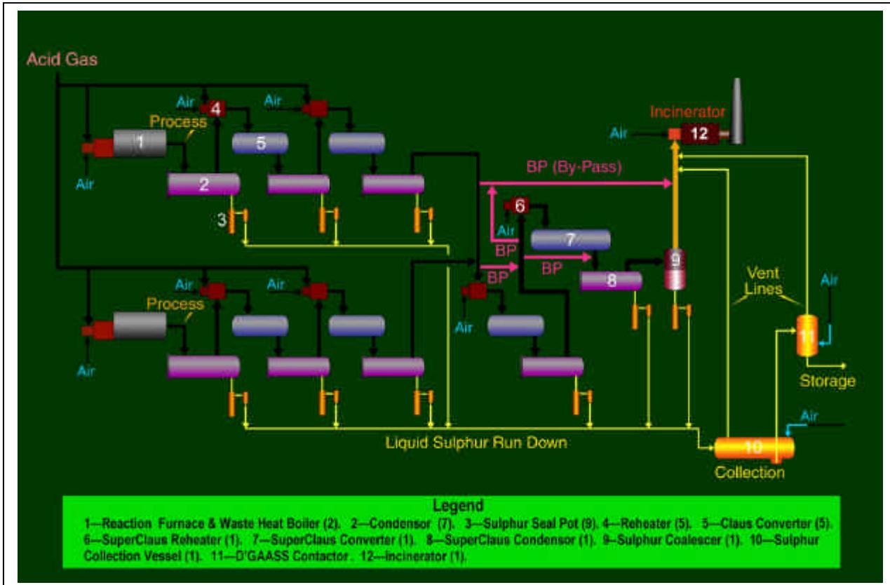
FIGURE 3 THERMALLY MAINTAINED PIPING IN UPGRADER SRU
