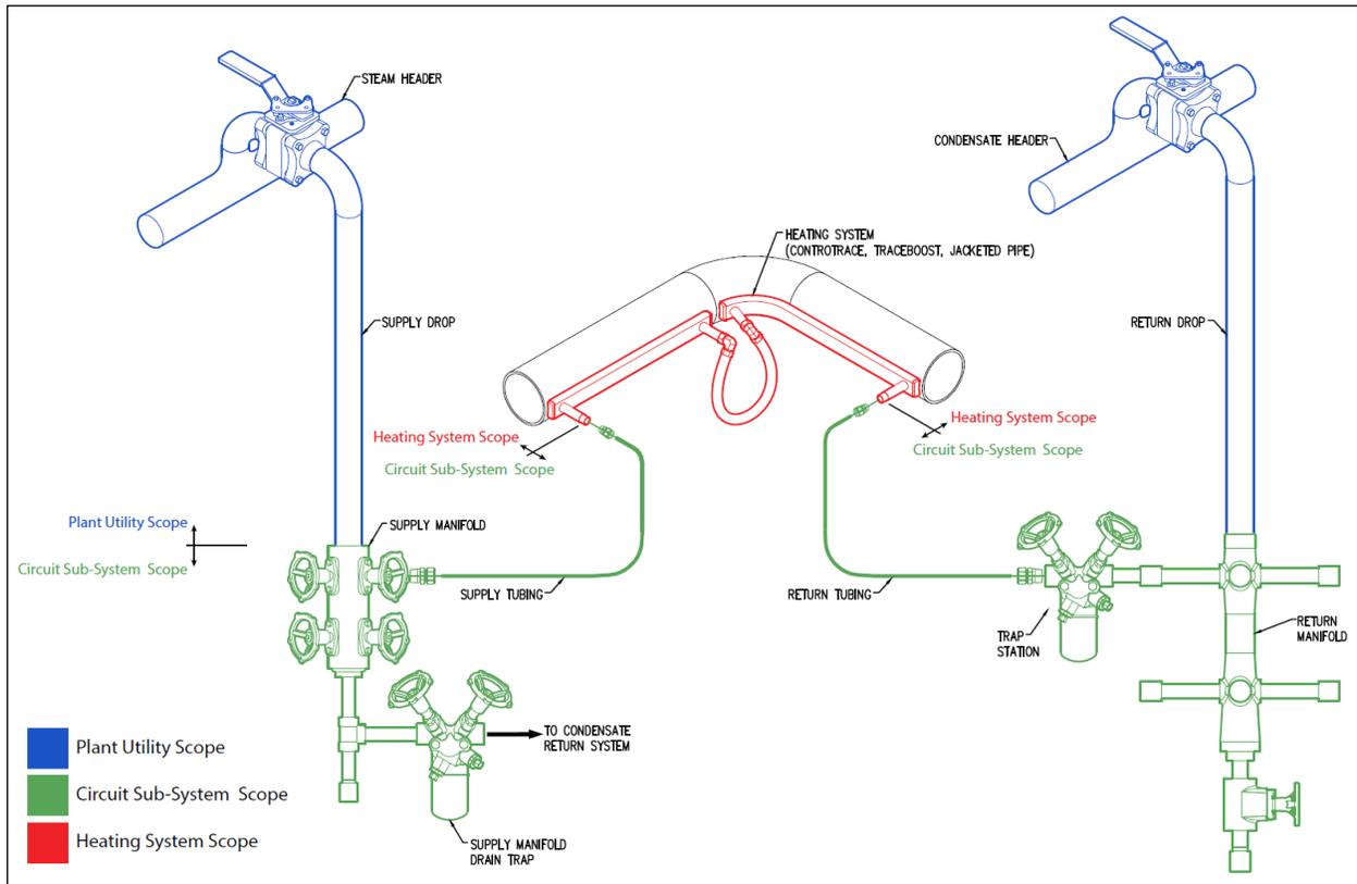
Figure 2: Components of a steam tracing circuit
