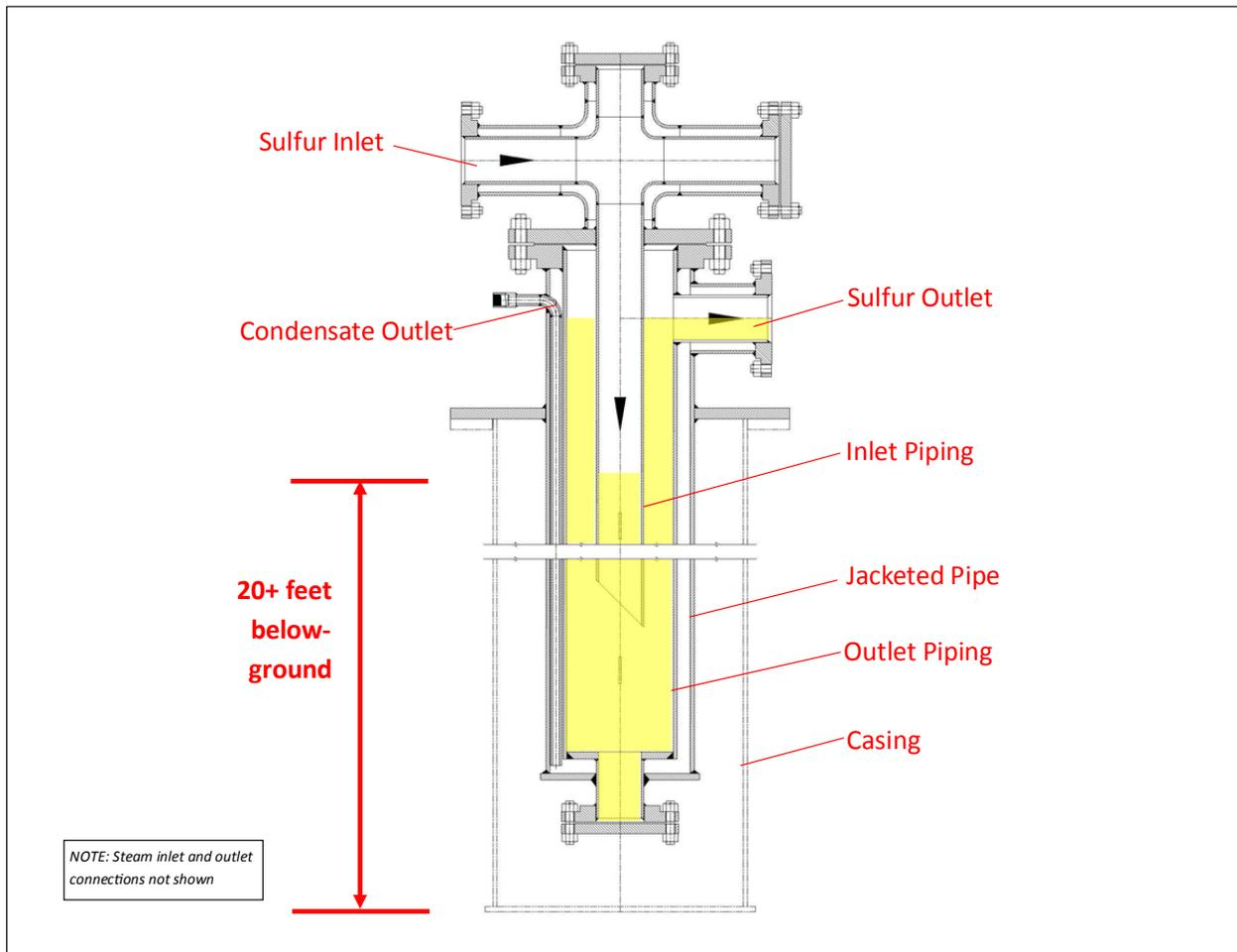
**Figure 2: Seal leg – traditional in-ground sulfur-sealing approach**
