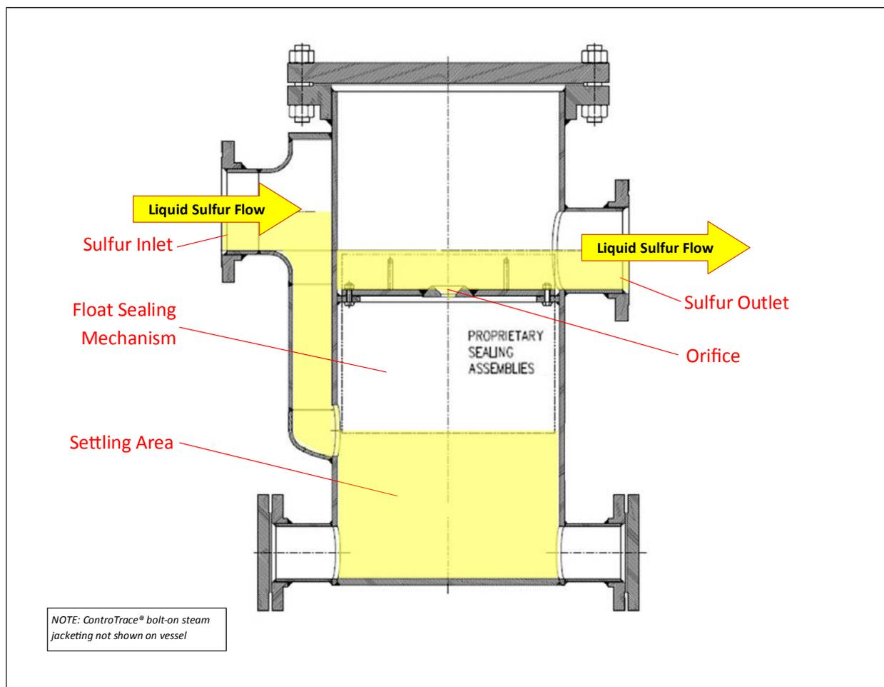
**Figure 9: SxSeal™ 2000 – improved above-ground sulfur-sealing technology**
