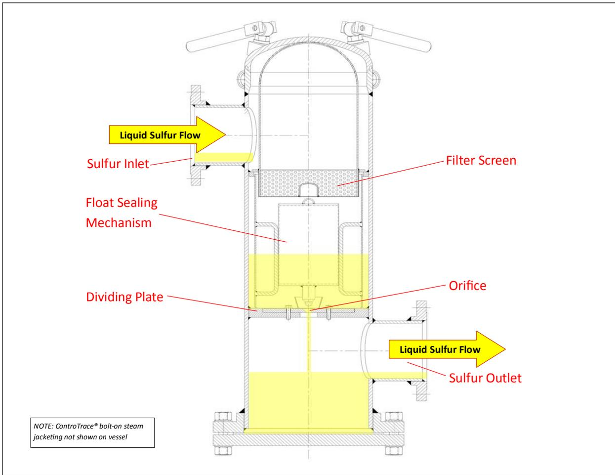
**Figure 3: S<sub>x</sub>Seal™ 1000 – conventional above-ground sulfur-sealing technology**
