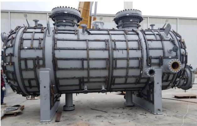
Figure 8. Horizontal vessel heated with ControTrace bolt-on heating panels.
