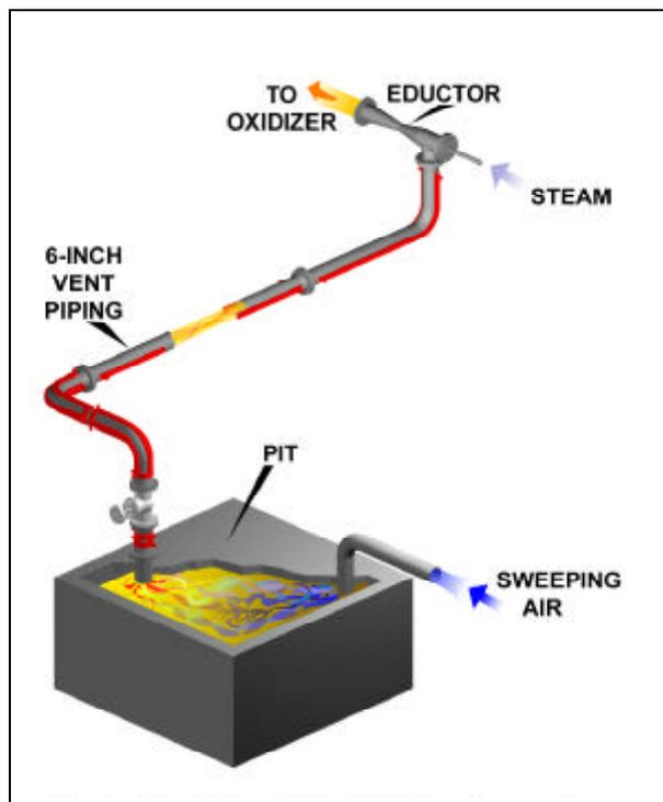
FIGURE 1 SULFUR PIT AND VENT PIPING LAYOUT
