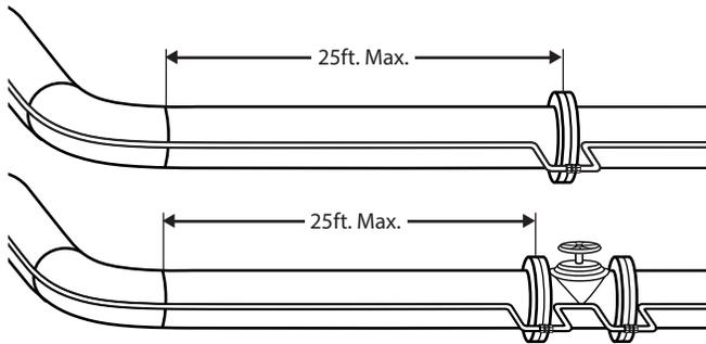
Fig. 4c: The maximum distance between a change in direction and an expansion loop is 25ft.
