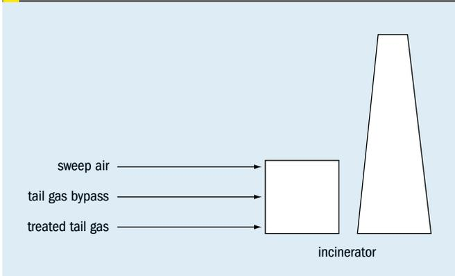
Fig 4: Routing 2 – combined treated tail gas and tail gas bypass, and independent sweep air line
