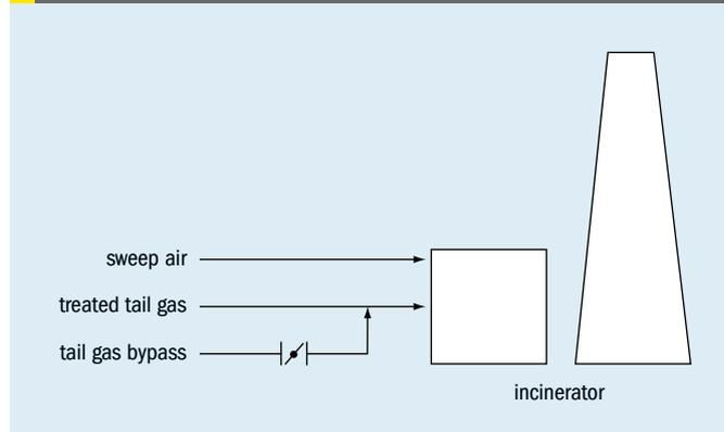
Fig 5: Routing 3 – treated tail gas, tail gas bypass and sweep air lines combined pre-incinerator
