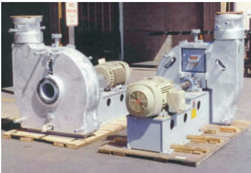
Fig. 7: Here Controls Southeast's ControHeat® type component jackets heat centrifugal blowers used in sulphur recovery at sulphur terminal.
