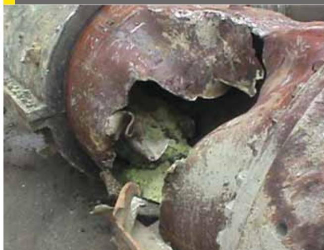
Fig 2: Tail gas line failure due to extreme corrosion
