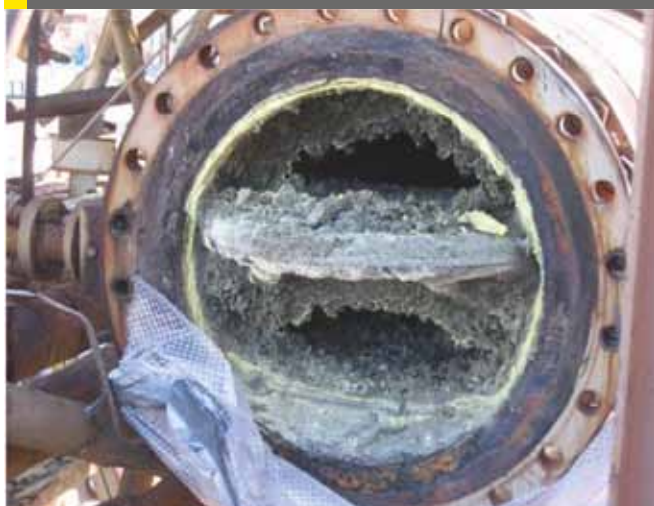
Fig 1: Tail gas line failure due to plugged diverter valve
