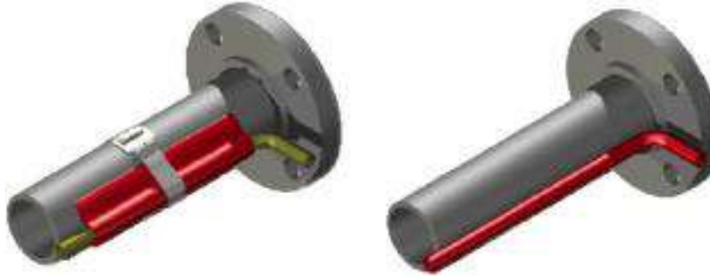
Figure 1: To-Scale drawing of TraceBOOST versus conventional steam tracing
