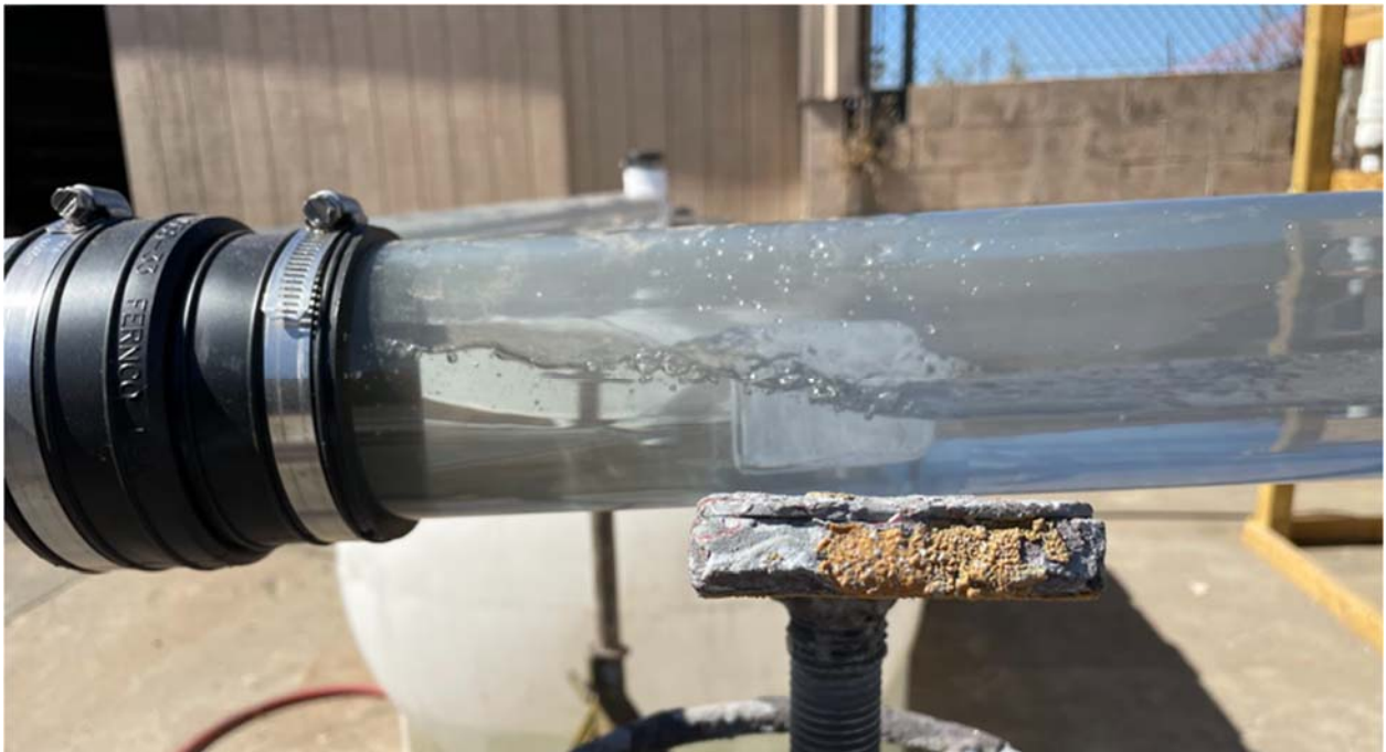
Example of liquid level rise at entrance to horizontal elbow fitting
