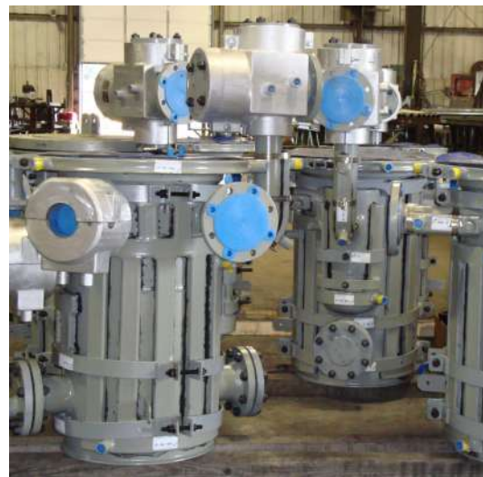
Jean Gaulin Refinery's S x Seal™ 2000 sulfur sealing devices, shown in production at CSI
