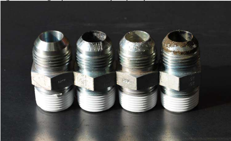
Figure 4: Damage inflicted to JIC adapters for Expts 10-11.
